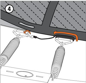
Wrap any remaining Connector Rope around the last D-shackle strap in the section.
