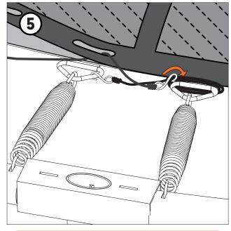
Continue with a new connector rope and repeat the steps until the Safety Net is fully secured.
