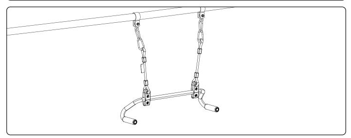
**NOTE:** Loosen bottom bolts until Monkey Swing has its handles parallel with the ground, then retighten the bolts.
