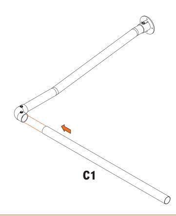
**WARNING:** Do not force any part too far into the Angled Joiner. This will block the part on the other side from connecting completely.
