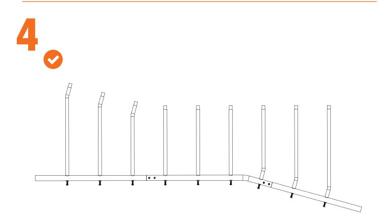
Make sure that the straight Climbing Bars are in the middle, and the angled Climbing Bars are in the either ends of the Climbing Rails, as indicated above.
