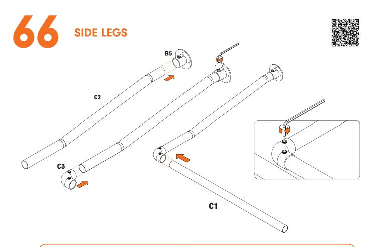
**WARNING:** Do not force any part too far into the Angled Joiner. This will block the part on the other side from connecting completely.
