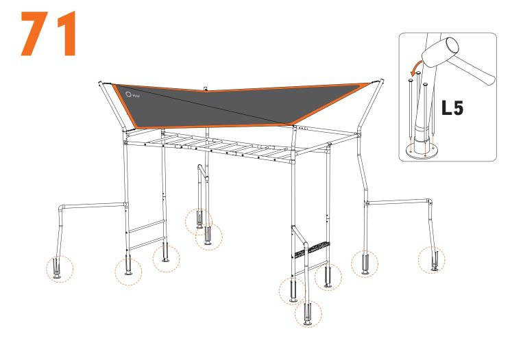
TIGHTEN ALL NUTS AND BOLTS AND ENSURE THE PARTS LOCK TOGETHER SECURELY.
