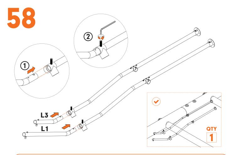
Double check to make sure all the pole's directions are accurately matching the image and that all holes line up with the grub screws before tightening.
