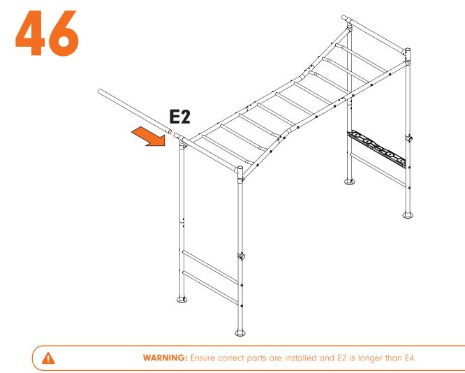
WARNING: Ensure correct parts are installed and E2 is longer than E4.
