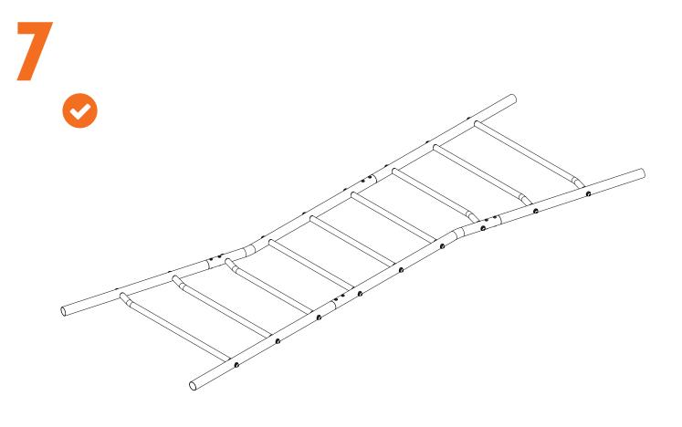
Once all of the climbing bars are loosely threaded into the climbing rails, tighten all of the bolts to make sure the climbing section is secure.
