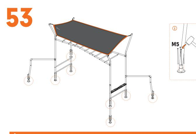
TIGHTEN ALL NUTS AND BOLTS AND ENSURE THE PARTS LOCK TOGETHER SECURELY.
