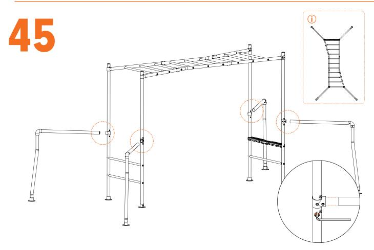
**Important:** Make sure the outer sections are positioned at 45°, relative to the climbing frame section.
