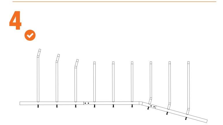
Make sure that the straight Climbing Bars are in the middle, and the angled Climbing Bars are in the either ends of the Climbing Rails, as indicated above.
