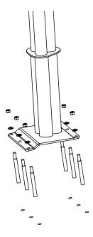
B. Insert the Telescoping Tube into the Base Plate.
