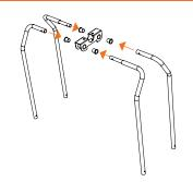
B. Insert a Top Bar (Male) and Top Bar (Female) into the Bushings on one side of the Top Connector.
