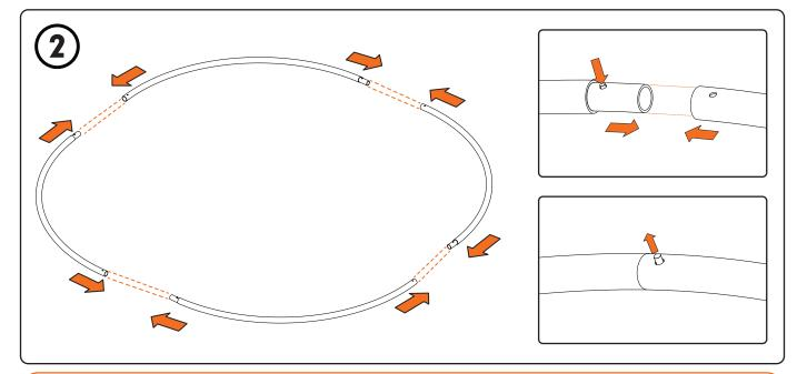
**WARNING:** Tighten all bolts and ensure all parts lock together securely.
