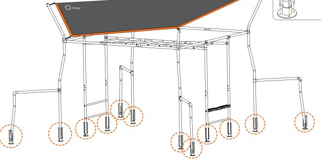
TIGHTEN ALL NUTS AND BOLTS AND ENSURE THE PARTS LOCK TOGETHER SECURELY.
